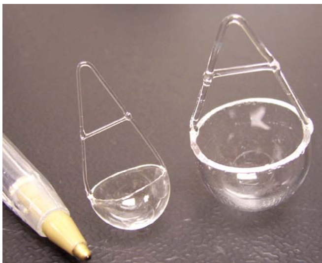
Figure 6.1: Quartz sample pans for a DVS-1 (left) and DVS-2 (right)
